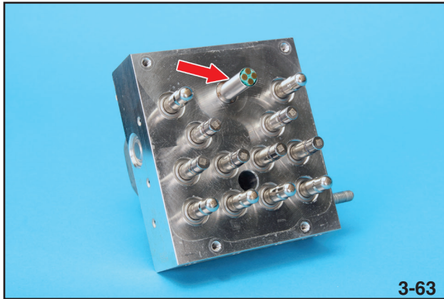
Brake Fluid Pressure Sensor - Internal
