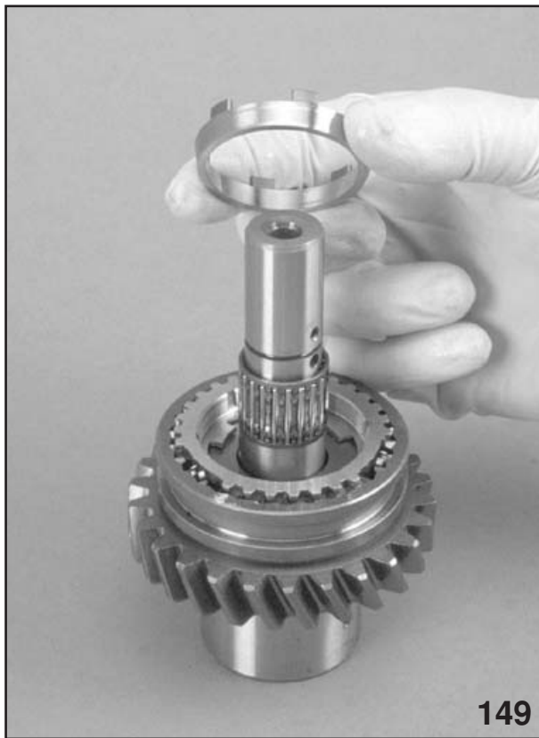
OUTER BAULK RING INSTALLED & INSTALLING SYNCHRONIZER CONE
