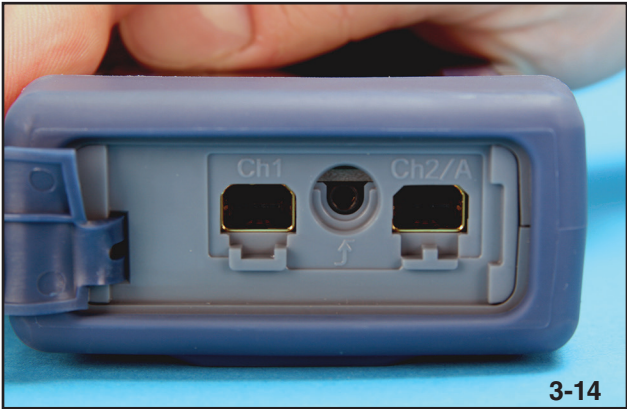
Channel 1, Channel 2 & Ground Connection
