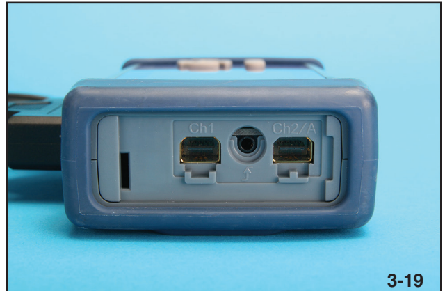
Oscilloscope Lead Connections
