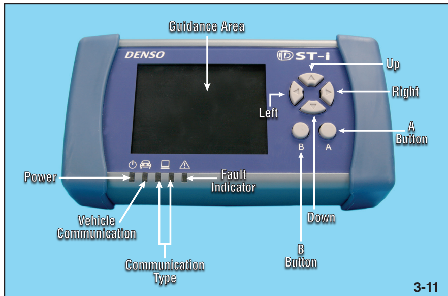
DST-i Controls and LEDs
