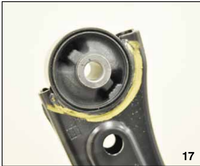
Cross Member Bushing, direction of gaps and solid material
