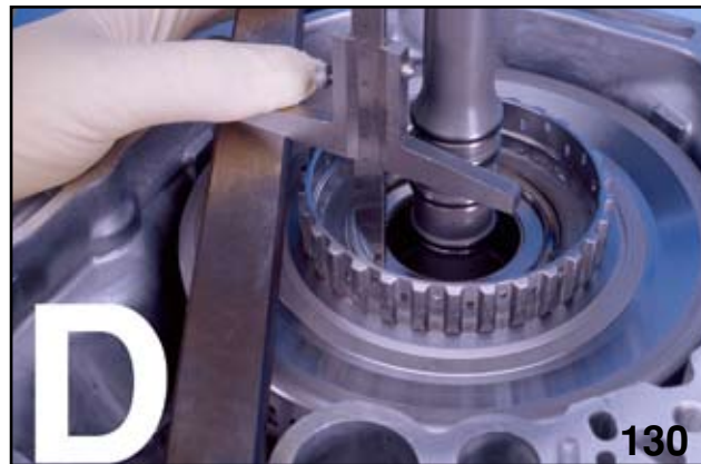
Mating Surface to Bearing Surface of the Front Sun Gear "D"
