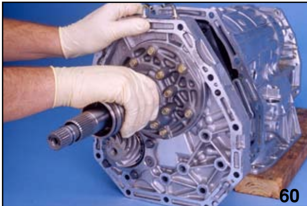
Separating Oil Pump Cover
