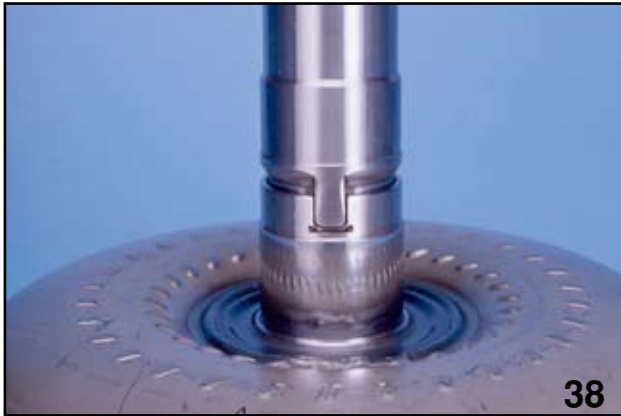
Separating Pump Drive
