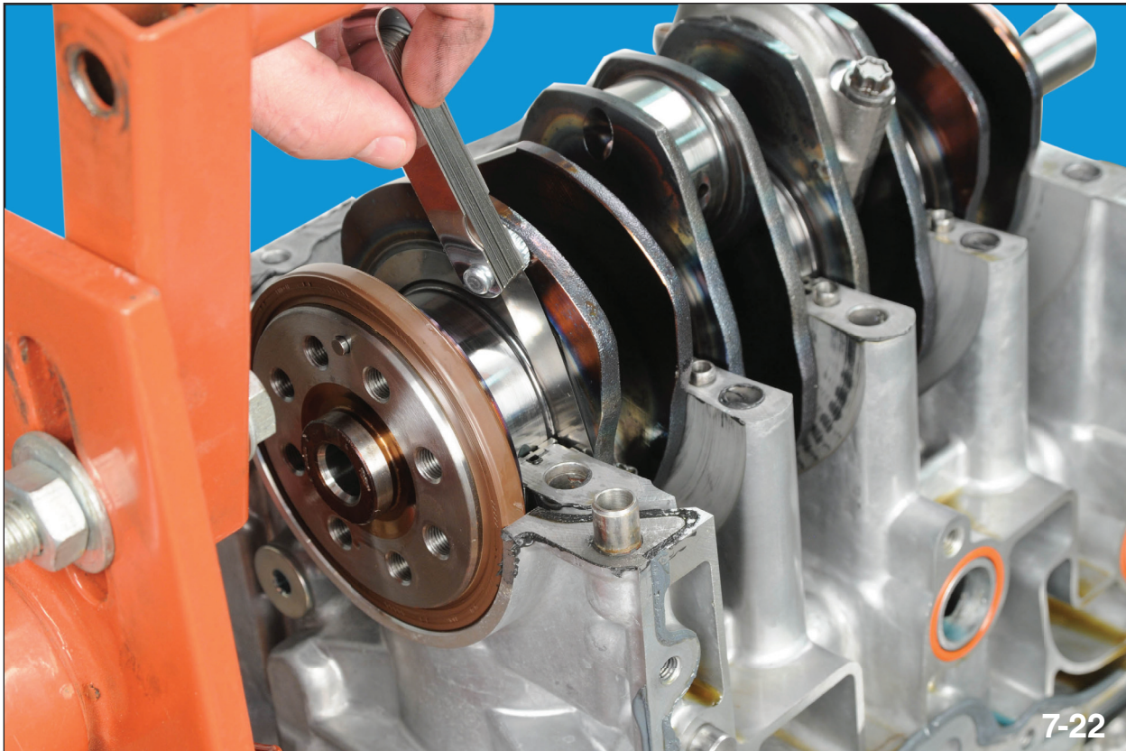
Checking Crankshaft Thrust Clearance
