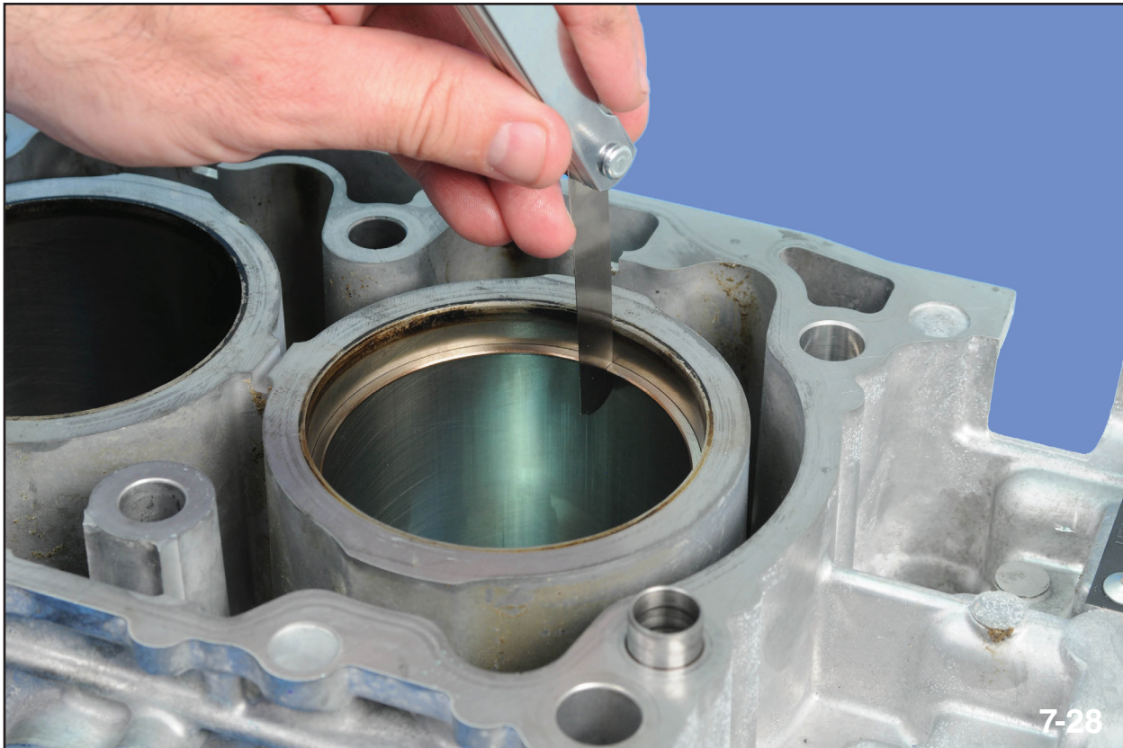
Checking Piston Ring End Gap
