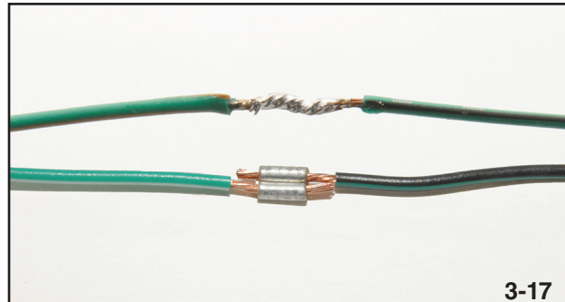
Solder vs crimping
