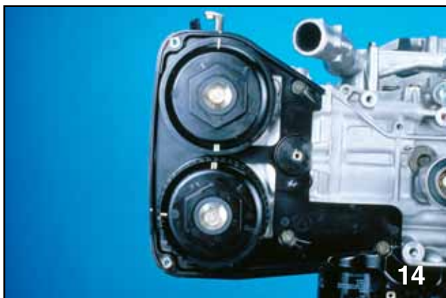
Camshaft Sprocket Timing Marks (Right Bank)
