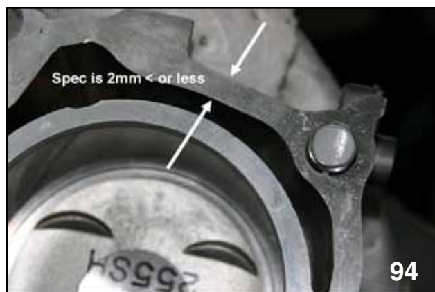
Scratch on Head Gasket Mating Surface (Flat)
