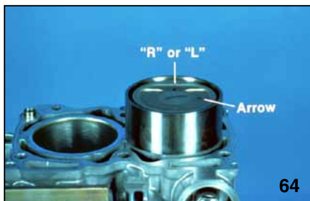
Piston Installation
