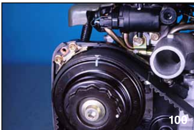
Intake Camshaft Sprocket Timing Marks (Right Bank)
