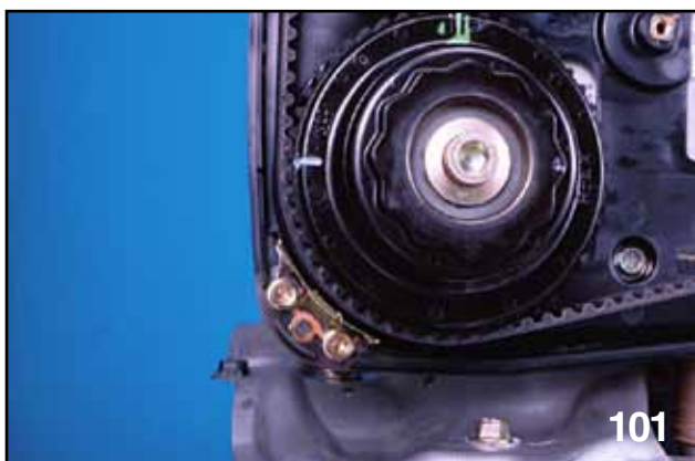
Exhaust Camshaft Sprocket Timing Marks (Right Bank)
