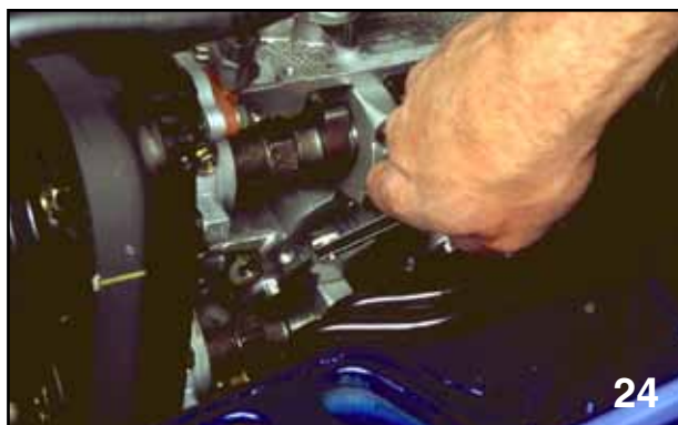
Checking Valve Clearance on the Car
