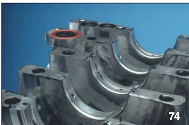
Main Bearing Oil Grooves
