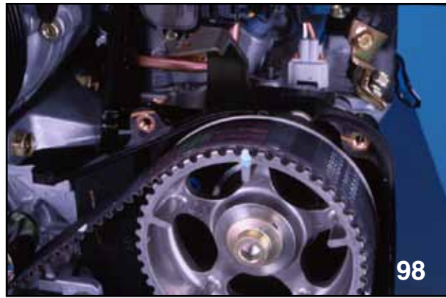
Intake Camshaft Sprocket Timing Marks (Left Bank)
