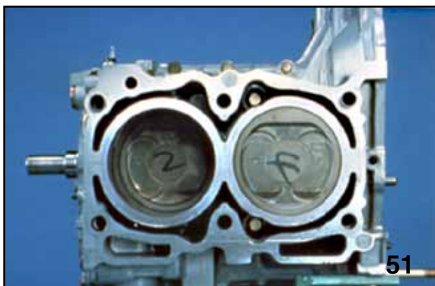
Crankcase Hidden Bolts (Left Bank)
