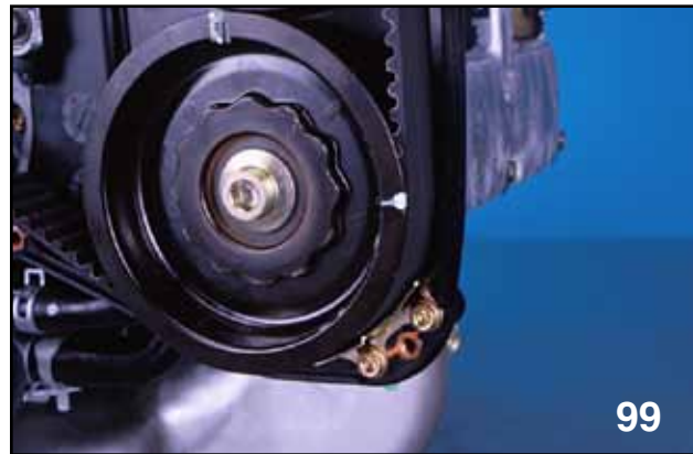
Exhaust Camshaft Sprocket Timing Marks (Left Bank)
