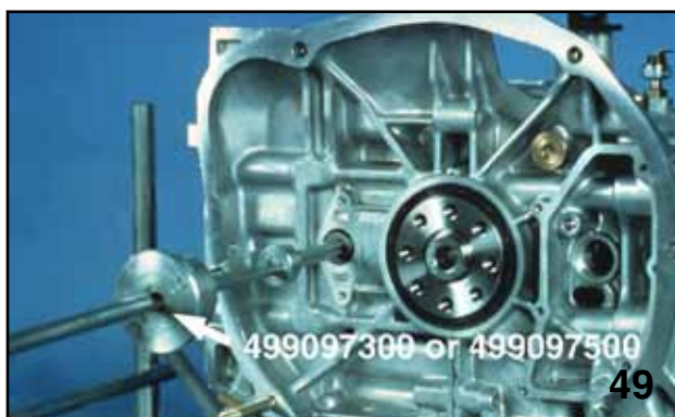
Piston Pin Removal
