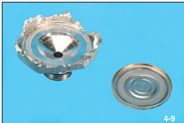
Legacy and Outback pressure sensor cutaway
